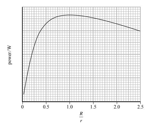
Determine whether maximum power is transferred to the motor.
