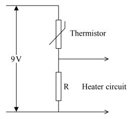
The heater circuit is connected across R and will switch on when the potential difference across it is above 5.5 V.
