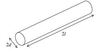
Sample A has a resistance  $R_{\rm A}$ . Sample B has a resistance  $R_{\rm B}$  and is twice the length and twice the diameter of sample A.
