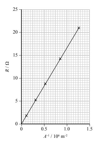
The resistivity of graphite is  $3 \times 10^{-5} \Omega$  m. Use the graph to draw a conclusion about the effect of adding clay to graphite.
