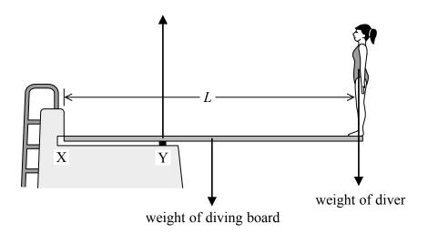
(a) The diving board has a length L of 3.6 m and is fixed at the end labelled X. It is supported at position Y which is 0.9 m from X. The diving board is uniform and has a weight of 390 N.
