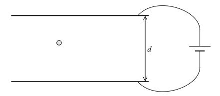
When the p.d. is 0 V the oil drop accelerates to terminal velocity. The p.d. is increased. It is observed that at a particular p.d. V the oil drop stops falling and remains stationary between the plates.
